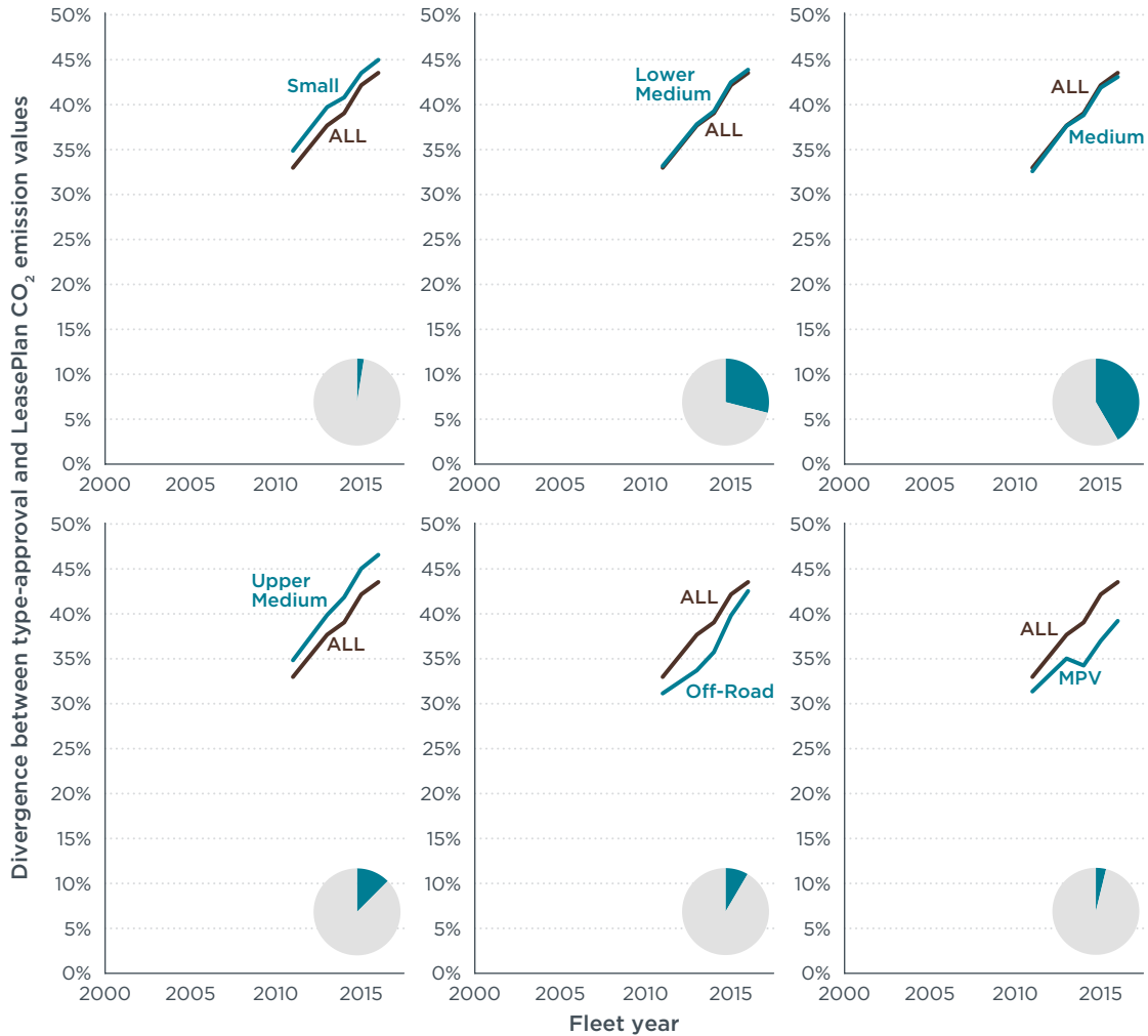
Figure 17. Divergence between type-approval and LeasePlan CO 2 emission values by vehicle segment. Pie charts represent the share of each segment in the dataset for fleet year 2016.
