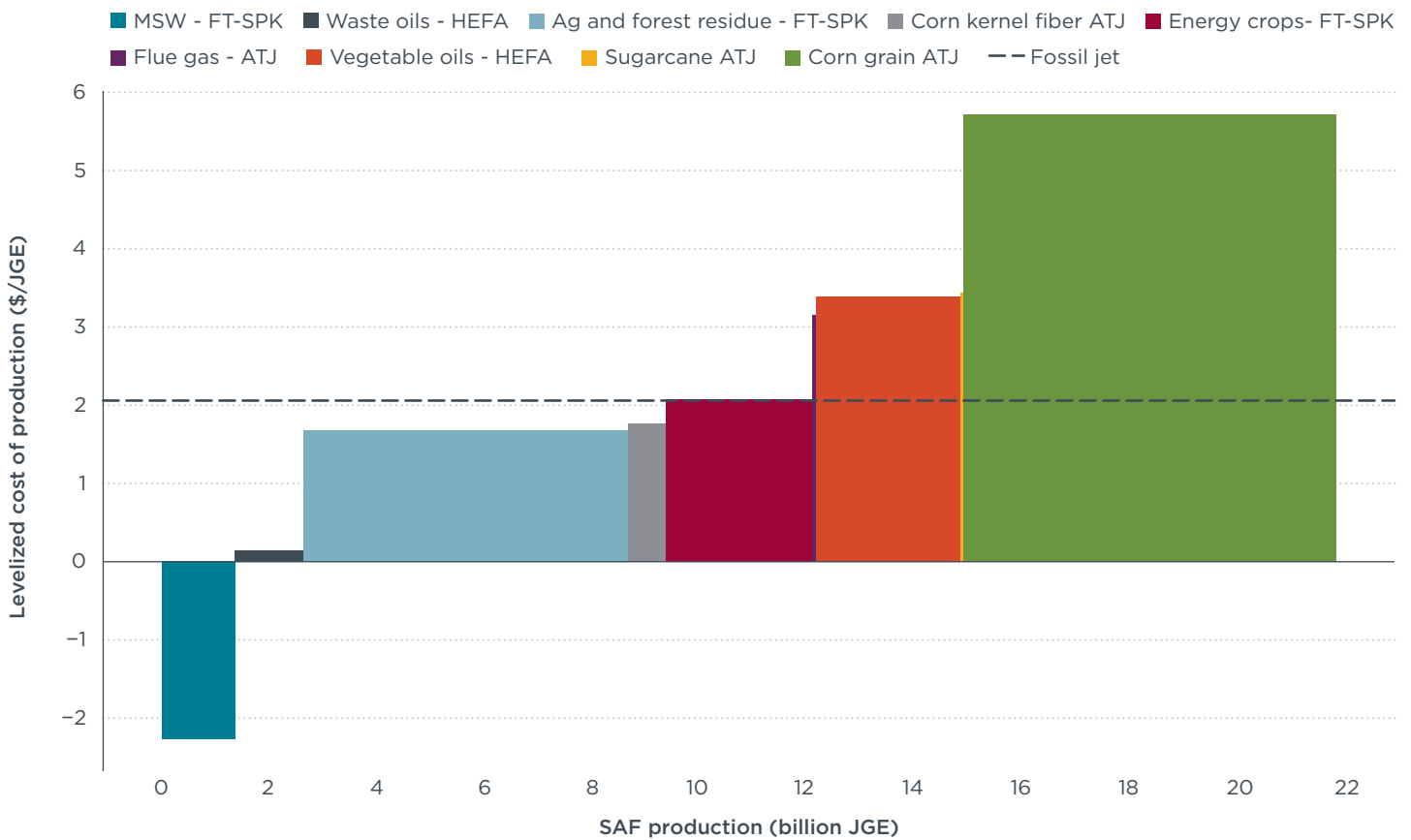
Figure 3. Estimated SAF production supply curve, relative to average cost of fossil jet fuel, adjusted for sustained 2022-2024 SAF policy incentives.
