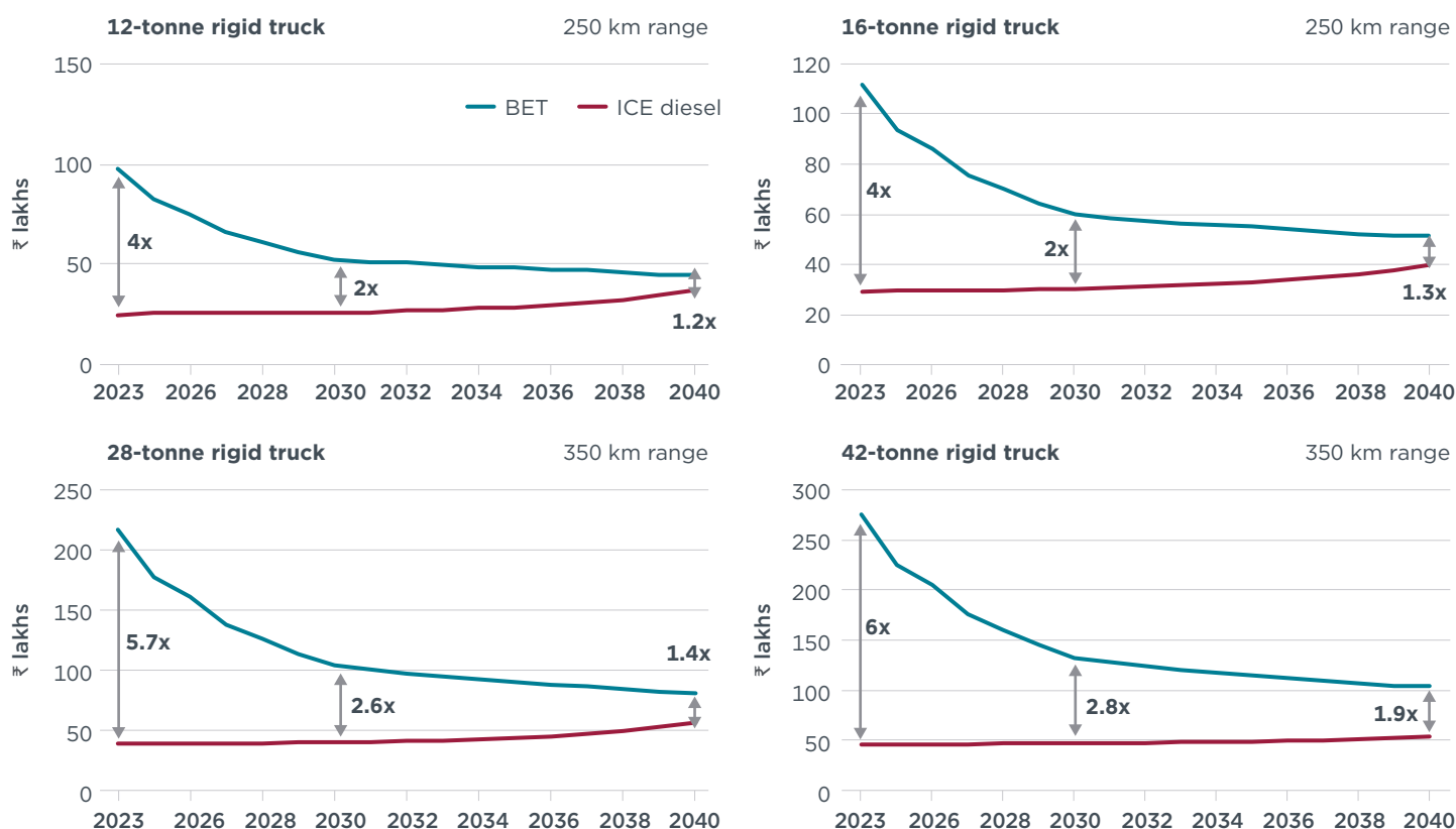
Figure 7 Upfront cost projections of BETs and diesel trucks assuming business-as-usual fuel consumption improvement
