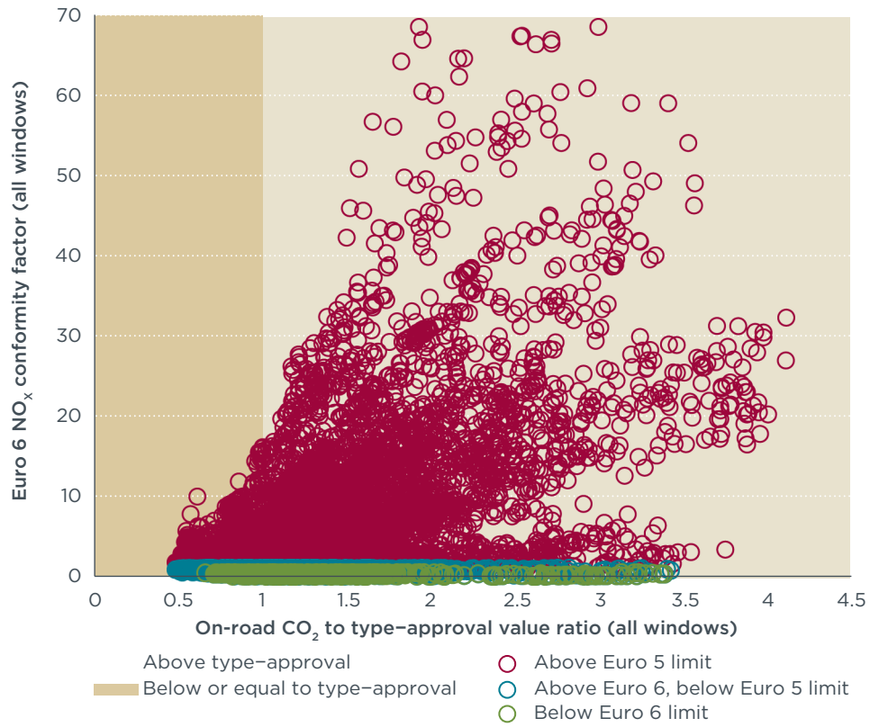
Figure 16: Scatterplot of NO x conformity factors and on-road CO 2 ratios (all windows)
