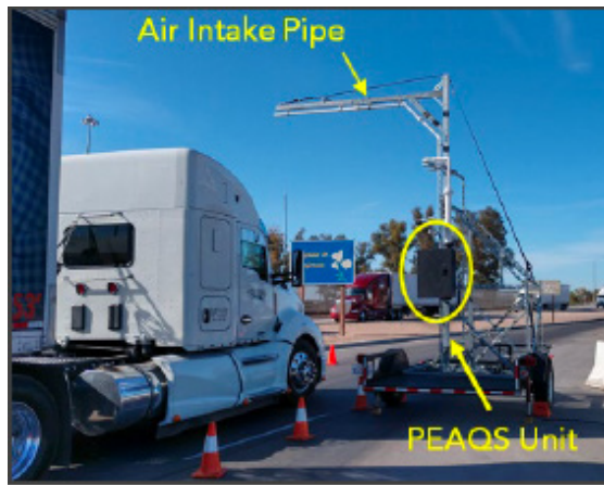
Figure 9. CARB's remote sensing system for diesel trucks. Source: California Air Resources Board (2021d)
