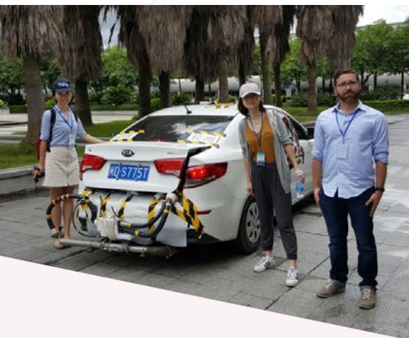
Emissions testing by ICCT staff in China using a portable emissions measurement system
