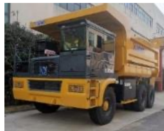
载货80-90吨，总重120-130吨 Cargo capacity 80-90 tons, weight 120-130 tons
