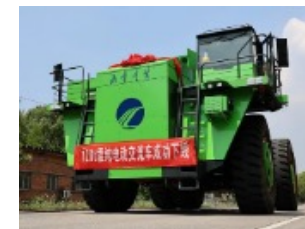
载货120-140吨级，总重220-240吨 Cargo capacity 120-140 tons, weight 220-240 tons
