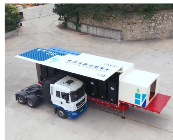
移动换电车/Mobile Battery Swapping Truck
