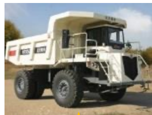
载货30-40吨，总重60吨 Cargo capacity 30-40 tons, weight 60 tons
