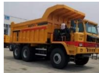
载货100-110吨级，总重150-160吨 Cargo capacity 100-110 tons, weight 150-160 tons
